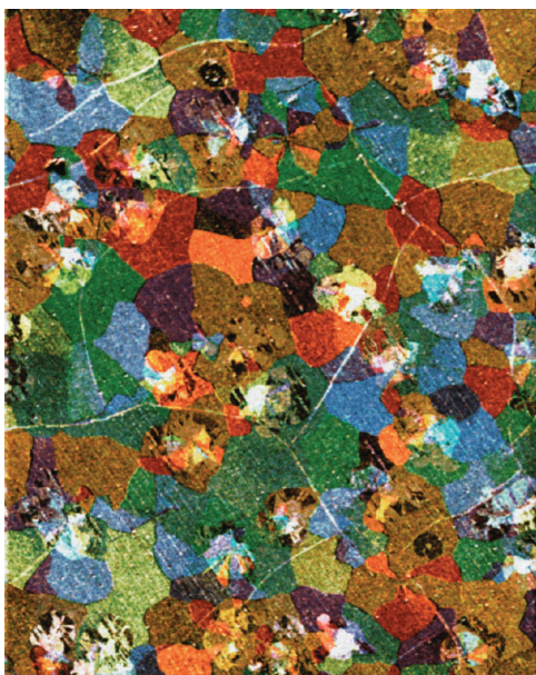
Figure 5. A 25 \mu\text{m} view, with color-coded orientations of graphene domains, each smaller than the copper grains, yet some visibly grown across the copper grain boundaries, marked out by white lines. (Courtesy of P. Huang and D. A. Muller, Cornell University.)
